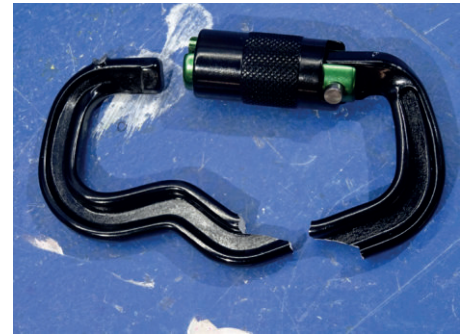
Broken aviation-sport carabiner after performed test
