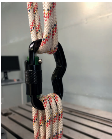
Test set-up of a carabiner test with „closed catch“
