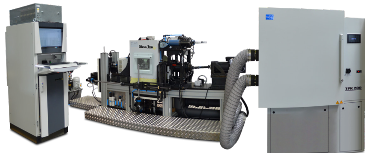
Friction torque determination for passenger car wheel bearings
