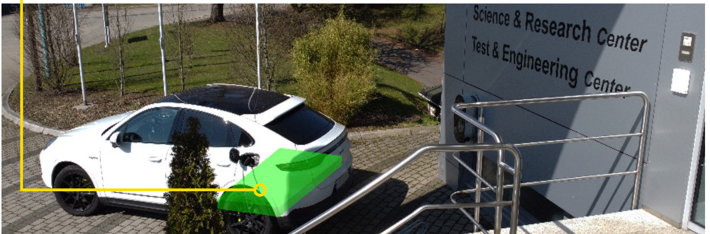
Exemplary setup of the test system with rolling worktable, here for testing a hybrid vehicle battery with six actuators
