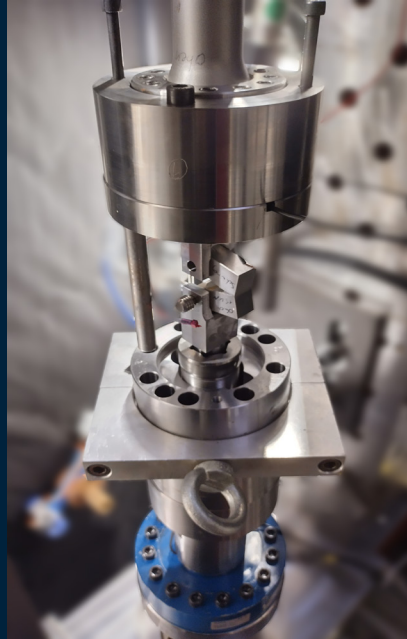
SincoTec hydrogen test cell with a CT sample
