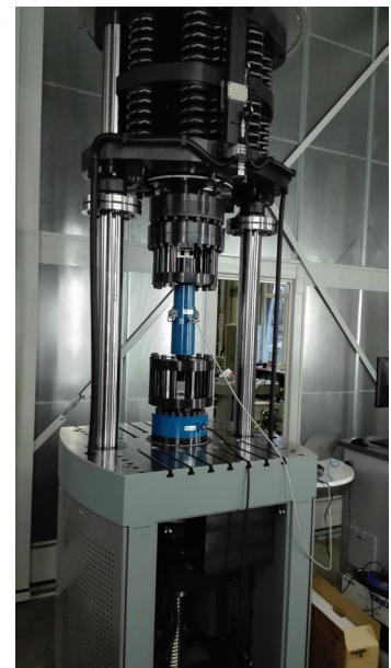
Calibration of a POWER SWING MOT resonance test system
