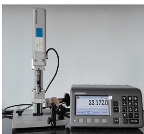
Calibration of a displacement transducer
