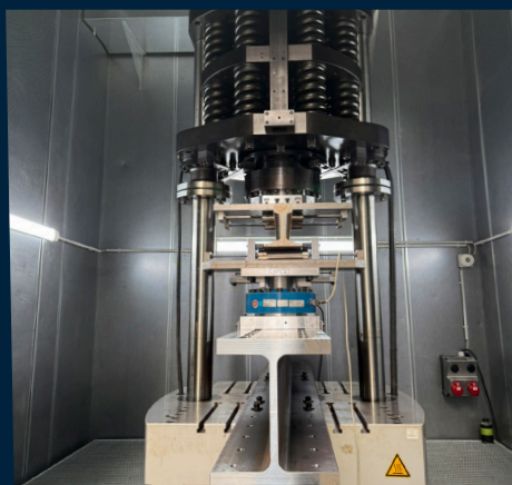
Figures: 4-point bending test on rails with a POWER SWING MOT evolution 600 kN
